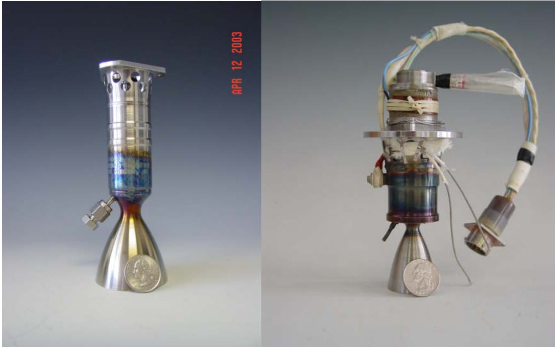
Figure 1. Left – 150 lbf 90% H 2 O 2 Thruster Shown Without Valve After Acceptance Test Right – 5 lbf Hydrazine Thruster Both Shown At Approximately Same Scale vs. US Quarter
