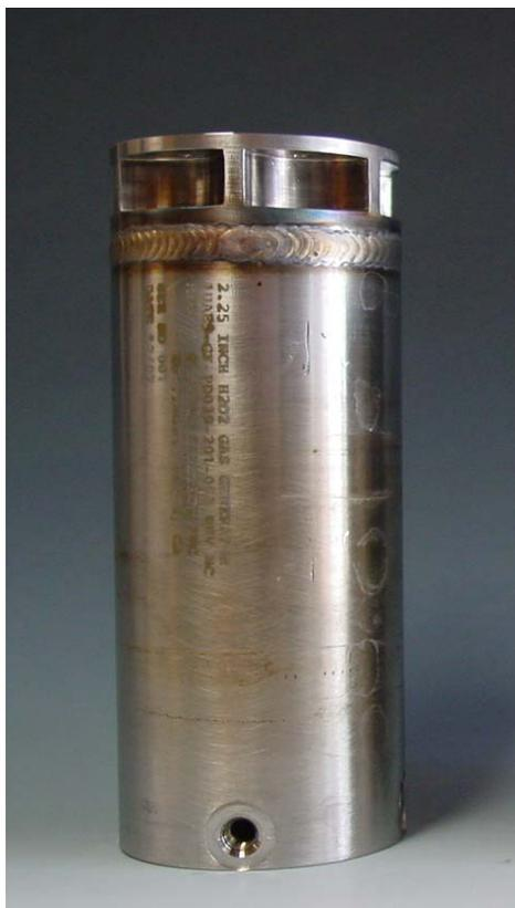
Figure 1 – 82-81% H<sub>2</sub>O<sub>2</sub> Gas Generator P/N: GK-PD039-201-003. GG is ~3 Inches (7.6 cm) in Diameter. Bottom is Exhaust End, One of the Four Instrumentation Ports are Shown In Photo.
