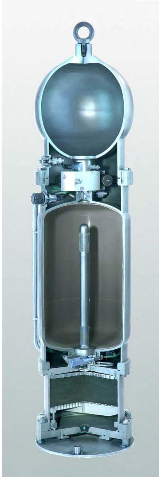
**Figure 11 – Cutaway View of the Liquid Hydrazine Gas Generator RESUS (Rescue System for Submarines) System for Emergency Ballast Displacement in Submarines. Hydrazine Mass per Gas Generator is Approximately 137 lbm. Gas Generator Manufactured by EADS Astrium and Deployed in German Submarines for More than 25 Years. (Ref. 25).**
