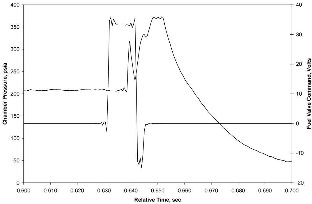
**Figure 8. Measured Chamber Pressure for Test 112303\_009**
