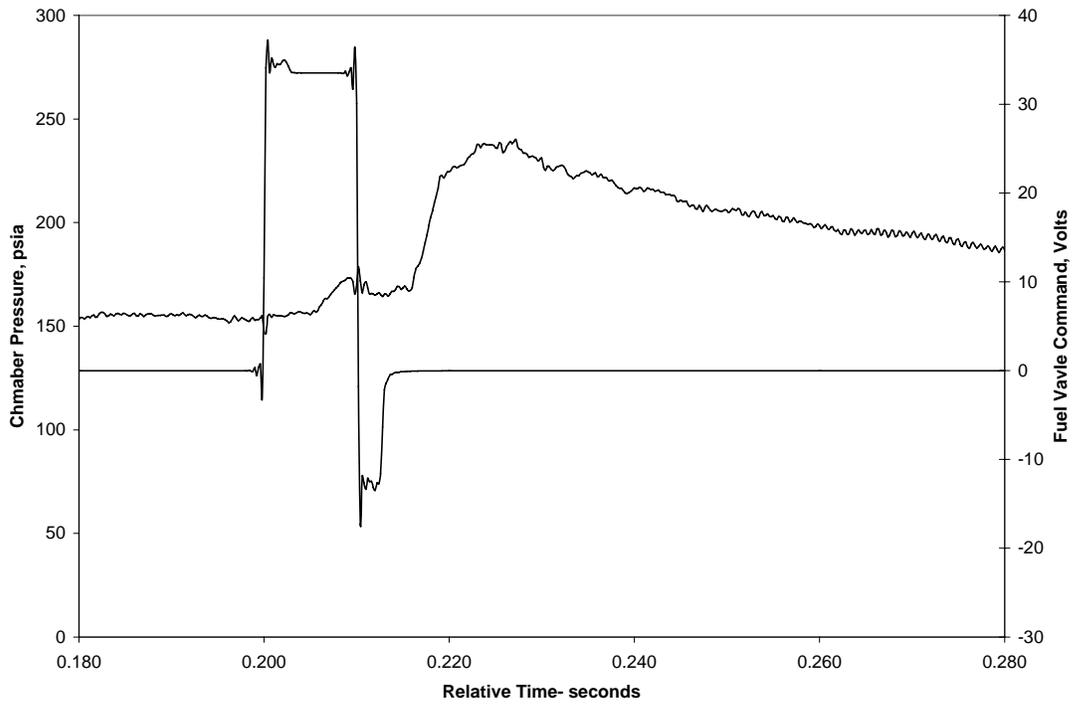
**Figure 5. Measured Chamber Pressure for Test 090303\_006 2<sup>nd</sup> Pulse**
