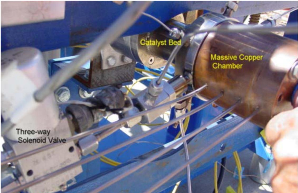
Figure 2. Details of Test Thruster
