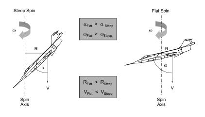
Figure 19. Distinction Between Steep and Flat Spin Modes
