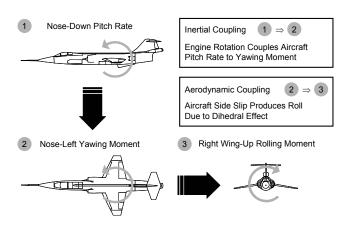
Figure 15. Aerodynamic-Inertial Coupling
