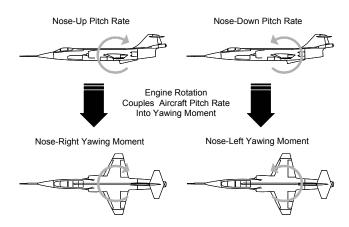
Figure 13. Turbojet Gyroscopic Pitch-Yaw Coupling
