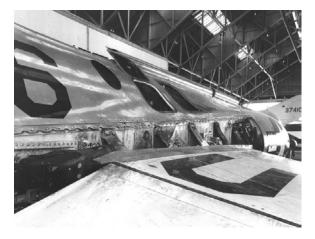
Figure 26. NF-104A Hydrogen Peroxide Damage
