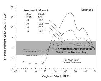
Figure 17. High Altitude RCS Pitch Control
