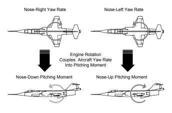
Figure 14. Turbojet Gyroscopic Yaw-Pitch Coupling
