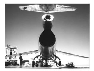
Figure 4. NF-104A Turbojet and Rocket Motor
