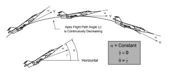
Constant Angle-of-Attack ( $\alpha$ ) is Maintained By Decreasing the Aircraft Pitch Angle at the Same Rate as the Continuously Decreasing Flight Path Angle ( $\gamma$ )
