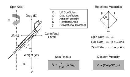
Figure 18. The Steady-State Spin
