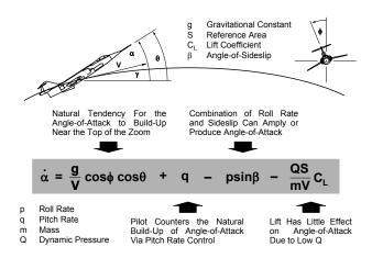
Figure 10. Factors Affecting Angle-of-Attack Rate
