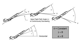
Holding the Aircraft at a Constant Pitch Angle ( $\theta$ ) Results in Angle-of-Attack ( $\alpha$ ) Build-Up Due to the Continuously Decreasing Flight Path Angle ( $\gamma$ )
