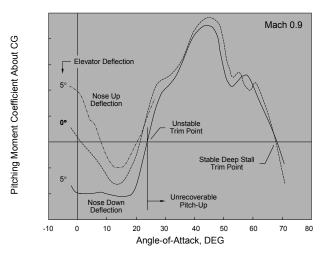
Figure 16. NF-104A Pitching Moment Characteristics
