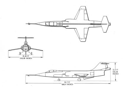
Figure 2. USAF/Lockheed NF-104A Aerospace Trainer (AST). Aircraft gross weight was approximately 22,000.
