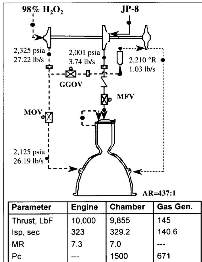
Figure 3: Representative Engine Power Balance
