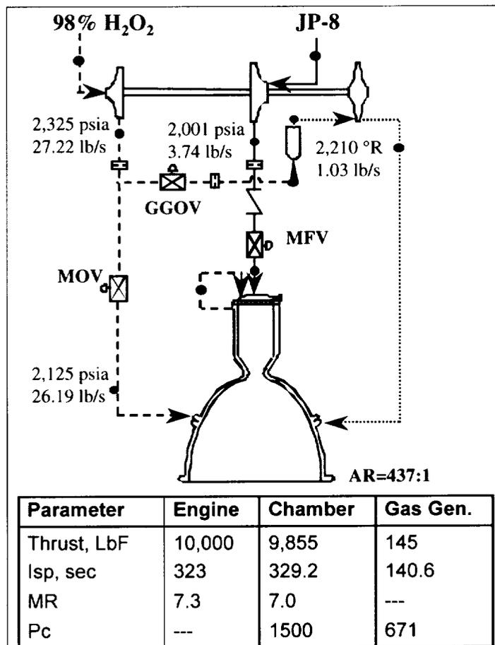
Figure 3: Representative Engine Power Balance
