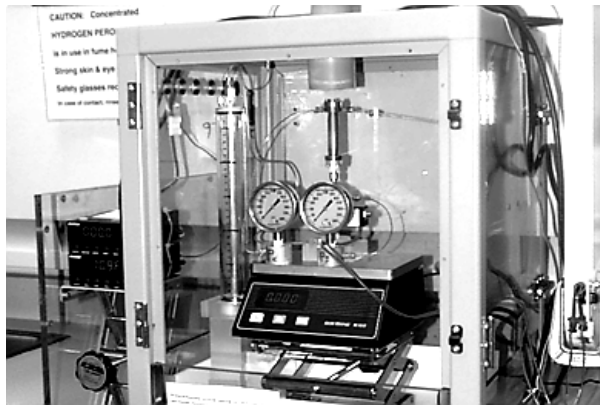
Figure 4. Thrust stand setup in benchtop safety enclosure.
