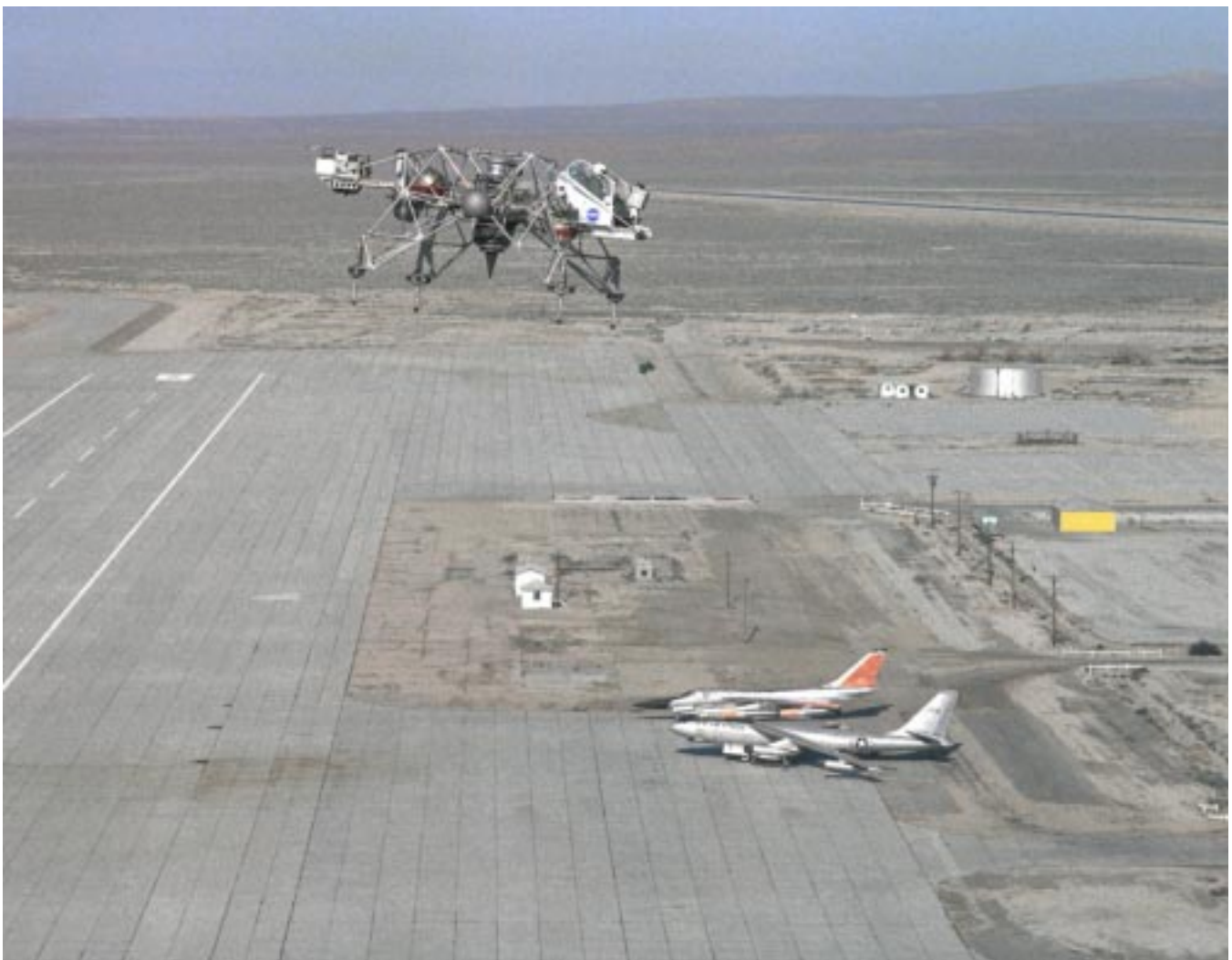
A Lunar Landing Research Vehicle is flown high over the South Base area of Edwards AFB during a test flight in 1965.
