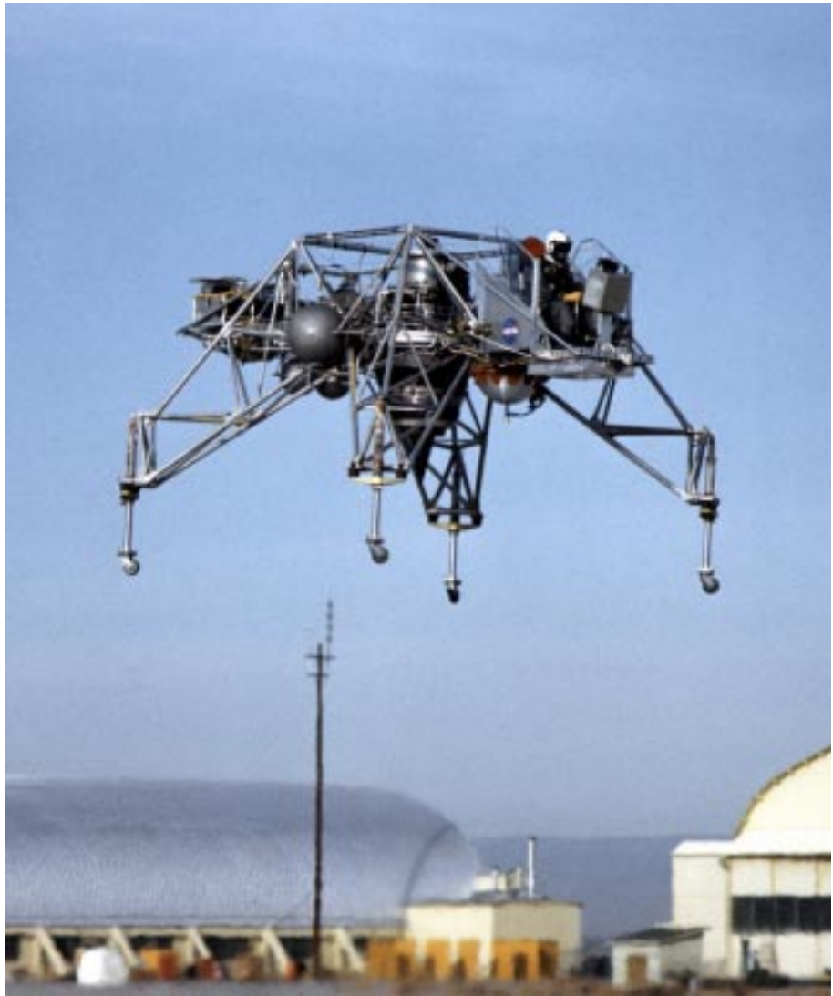
A Lunar Landing Research Vehicle is maneuvered during a test flight in 1964.
