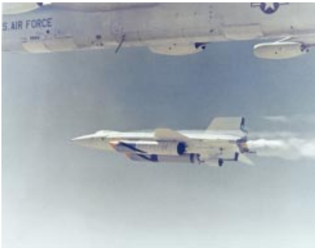
X-15 No. 2, with a white ablative coating and twin external fuel tanks, drops away from NASA's B-52 carrier aircraft. The aircraft, in this configuration, set the world's speed record of 4,520 mph for winged aircraft.
