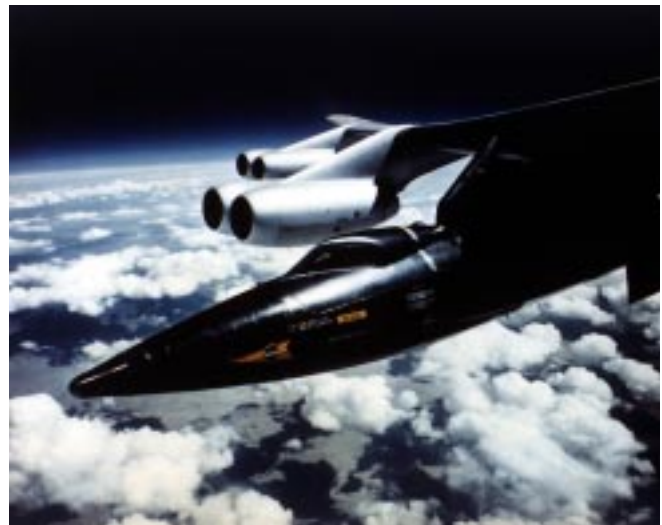
An X-15 hangs from a pylon beneath the right wing of NASA's B-52 carrier aircraft as the moment nears to drop the rocket-powered aircraft on a high-speed research flight
