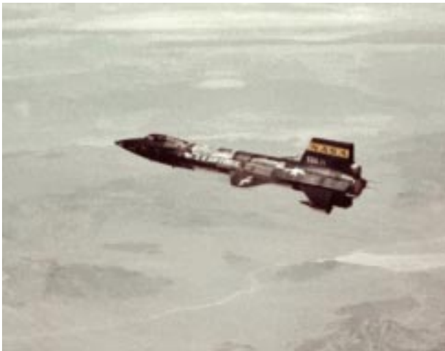
X-15 No. 2, with a dummy ramjet mounted on the lower ventral fin, is pictured at the beginning of a research flight following an air drop from NASA's B-52 carrier aircraft.
