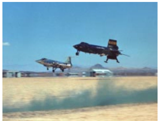
An X-15, with landing skids and nose wheel down, nears the dry lakebed at Edwards AFB following a research flight, while accompanied by a NASA F-104 chase aircraft.
