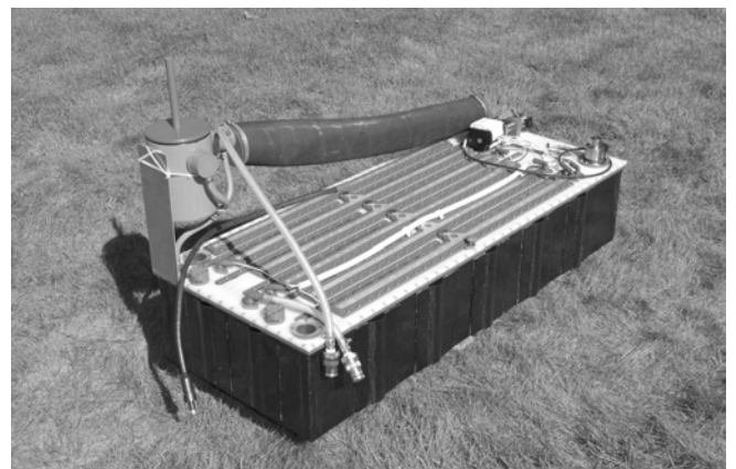
Fig. 4. Battery box (cell stack).
